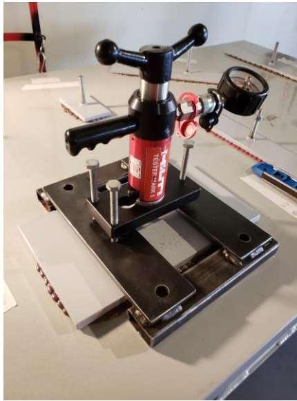
Figure 4: Hilti Mark 5 tester and Steel Bridge
