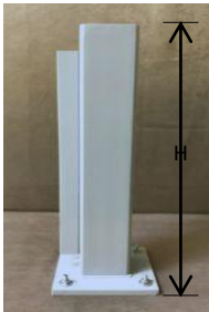
Upright Floor Mount Pedestal HSS4"x4", HSS 3"x3" MEP FLR-T4S Base 8"x8" – 1/2" Plate
